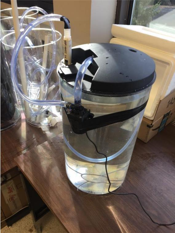
Fig 4. The mark one prototype of the original design to test the power of the water pumps to ensure it was sufficient to move the amount of water required to create a current.
